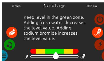
The green zone in the center area of the gauge should be targeted for optimal performance.
